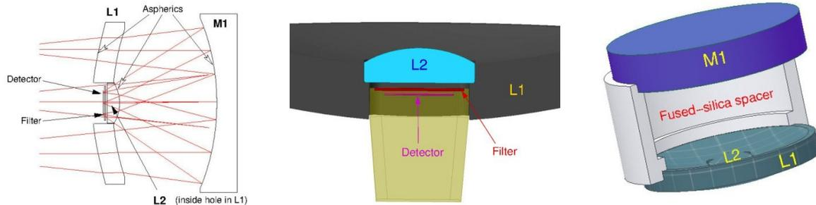
**Figure 3** Rays tracing and views of the Wonder-Camera including details of the L1-L2 interface and a possible T-invariant mount.
